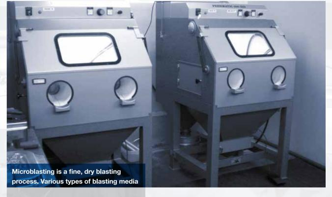
with precisely defined grain sizes and geometries are blasted onto the surface of the workpieces using compressed air. During this process the microtopography is specifically influenced. Textures are removed from the surface, it is cleaned, compacted and, if necessary, tribologically effectively modified.
